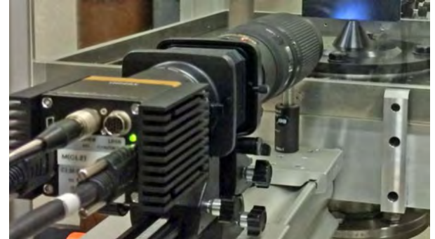
Figure 1. Jet flow experiment with Microvec LF-PIV camera
